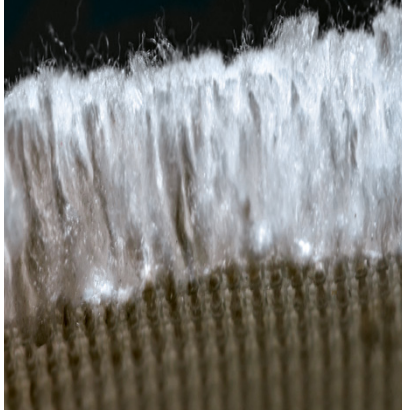
Polyamide pile cloth on polyester fabric
