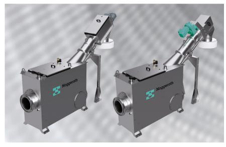
Equipment for the fine screening of wastewater in inlet has been part of the standard range of the brand Noggerath® of Passavant-Geiger since 1988. Our compact and robust spiral sieves are availible integrated in a stainless steel receiving tank with and without dewatering / compacting zone. The liquid flows into the sieve basket, which is open on the inlet side. Solids with a larger diameter than the hole / gap width are retained. A continuous layer of
