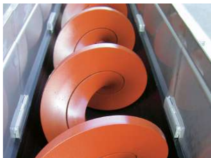
Spiral guided by PE-UHMW wear Lining
