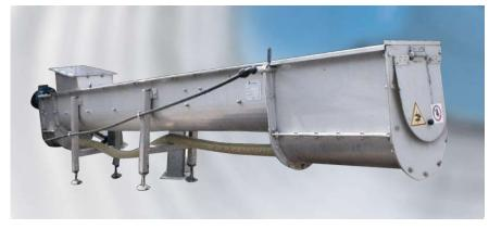
The Apseptence Group offers you the Noggerath® Spiral Compactor SCD with its centrepiece, the shaftless spiral which reliably conveys, dewaters and compacts even problematic materials – e.g. conbining fibres or grit – without clogging. Size, length and installation angle can optimally be tailored to meet indivi-
