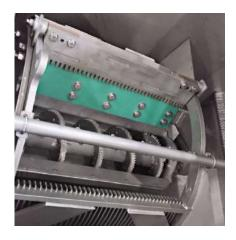
With the Passavant® Rotating Bar Screen RBS the Aqseptence Group offers a compact system for automatic waste water treatment.
