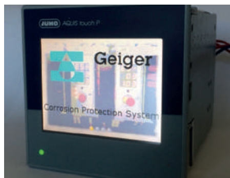
Fig. 5: Potential controller with operating program start-up notification
