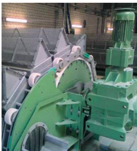
Centre Flow Travelling Band Screen with Roof-Shaped Mesh Panel Design
