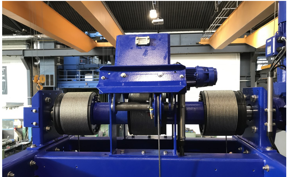
Polyamide hose drums at Geiger® Cable Operated Bar Screen
