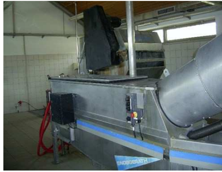
Paternoster screen with screenings washing
