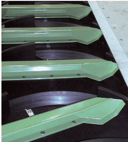
Picture on the right: Geiger® MultiDisc® Screen – Fish Protection Systems
